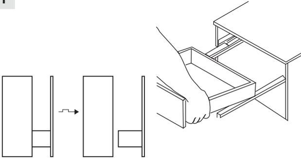
Pull out the drawer to its full extension by gently gripping the release levers on both sides and pull the drawer off the runners at the front.
